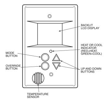
Fig. 2 — Thermostat Front Panel
